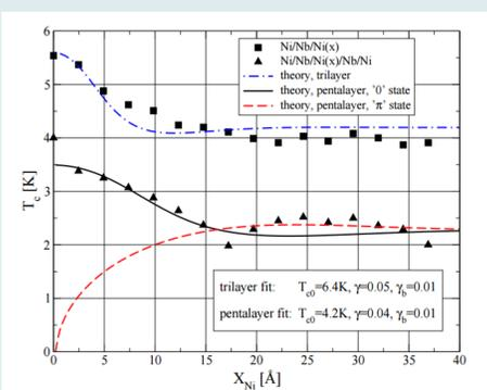
**Fig. 3.** (From [3]) Critical temperature as a function of Ni thickness for a trilayer Ni/Nb/Ni and pentalayer Ni/Nb/Ni/Nb/Ni; exhibits re-entrant superconductivity; data fit to linearized Usadel equation, with spin triplet component.
