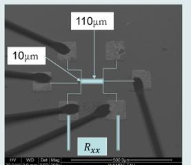
**Fig. 4:** ESEM micrograph of a typical sample
