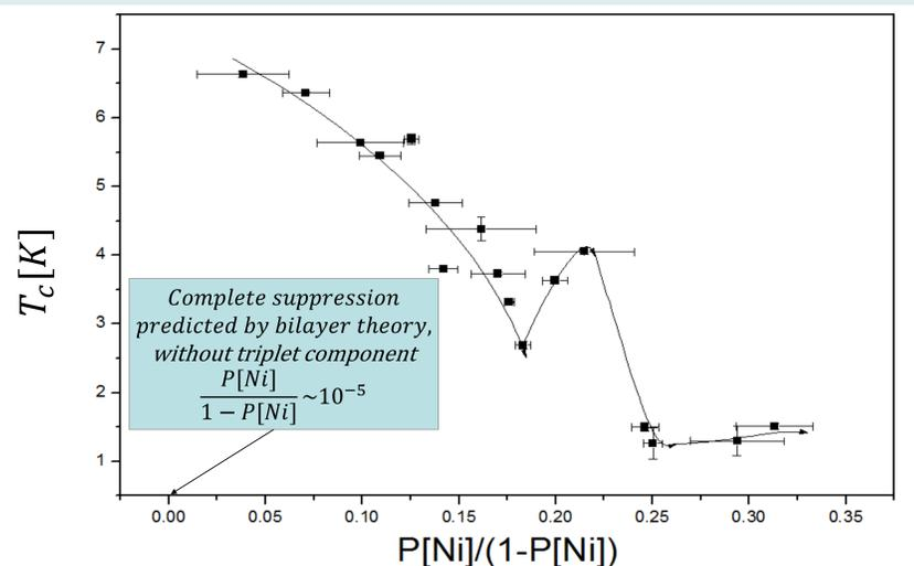
**Fig. 5:** Critical temperature as a function of relative volume concentration of Ni in granular SF structures; exhibits non-monotonic behavior.
