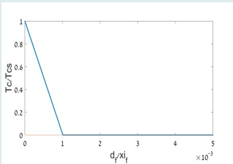
**Fig. 1. SF Bilayer:** Monotonic decay of  $T_c$  as a function of  $\frac{d_f}{\xi_f}$ . Calculated according to linearized Usadel equation, simplified for a thin S layer [1]. Note: For Ni/Pb system, superconductivity is suppressed for F layers  $\sim 0.01\text{\AA}$
