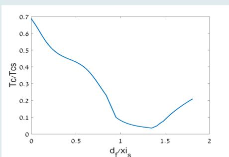
**Fig. 2. F/S/F Trilayer:** Example of re-entrant behavior of  $T_c$  as a function of  $\frac{d_f}{\xi_s}$ . Calculated according to linearized Usadel equation [2], including Cooper pair triplet component.
